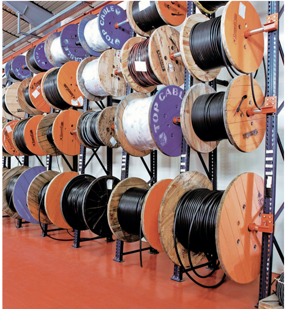
Racking for reels Racking for reels is designed to provide a simple and safe solution for the storage of cylindrical items using a metal axle.
