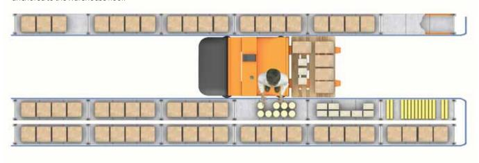
Each model of machine needs its own type of guide rail and a distinct aisle width. The aisle width is defined by the distance between the guide rails and the distance between the load levels.
