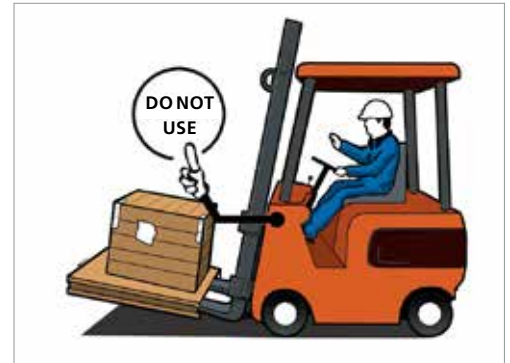
Forklift not operational.
