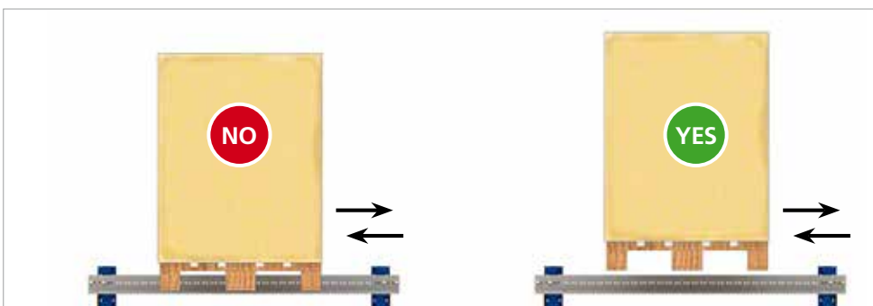
Figure 10. Do not drag the pallets along the rails. Lift and reposition.
