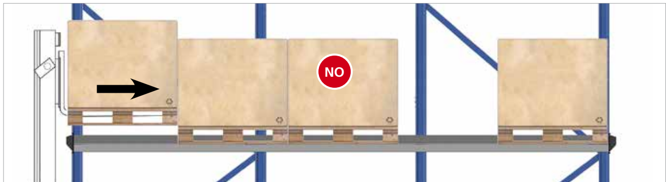
Do not push the pallets with the forklift. Lift and reposition.
